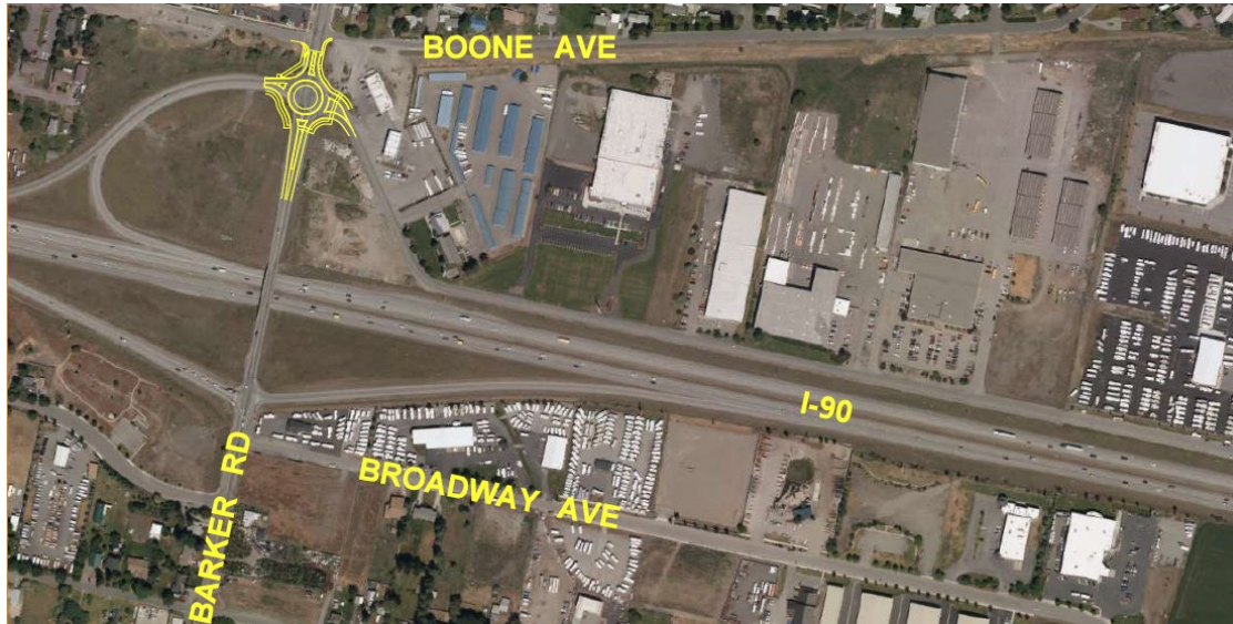
Figure 8. Barker Road/I-90 westbound ramp intersection – revised Interim Concept
